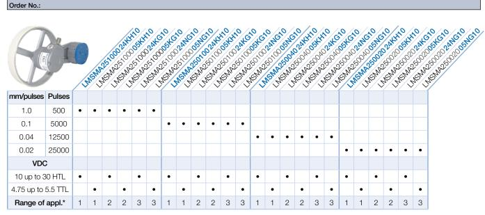
\* Range of application measuring wheel U = 500 mm
